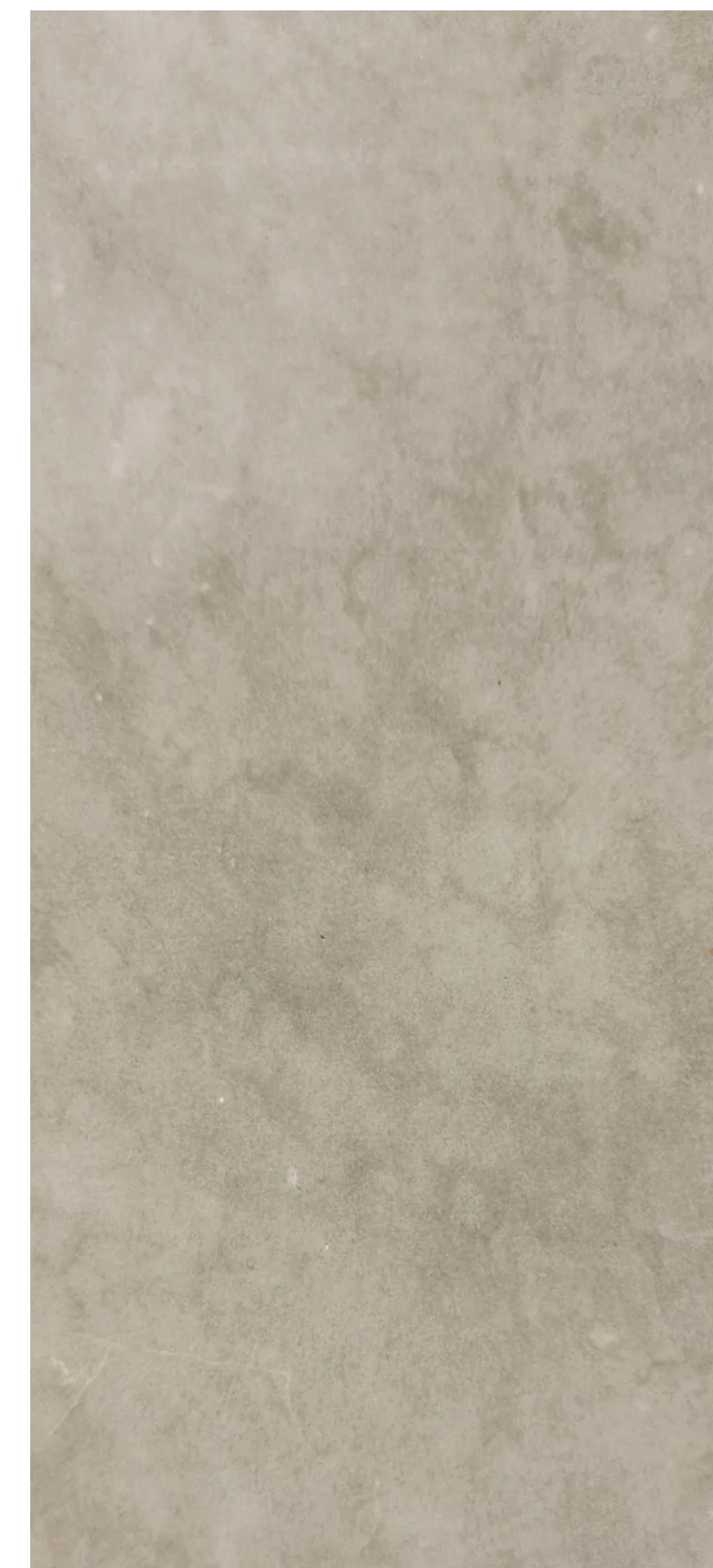
PORTLAND CEMENT PLASTER INTEGRAL COLOR - LIGHT GREY - BROWN FINE SAND FLOAT WITH HAND TROWEL BURNISH
