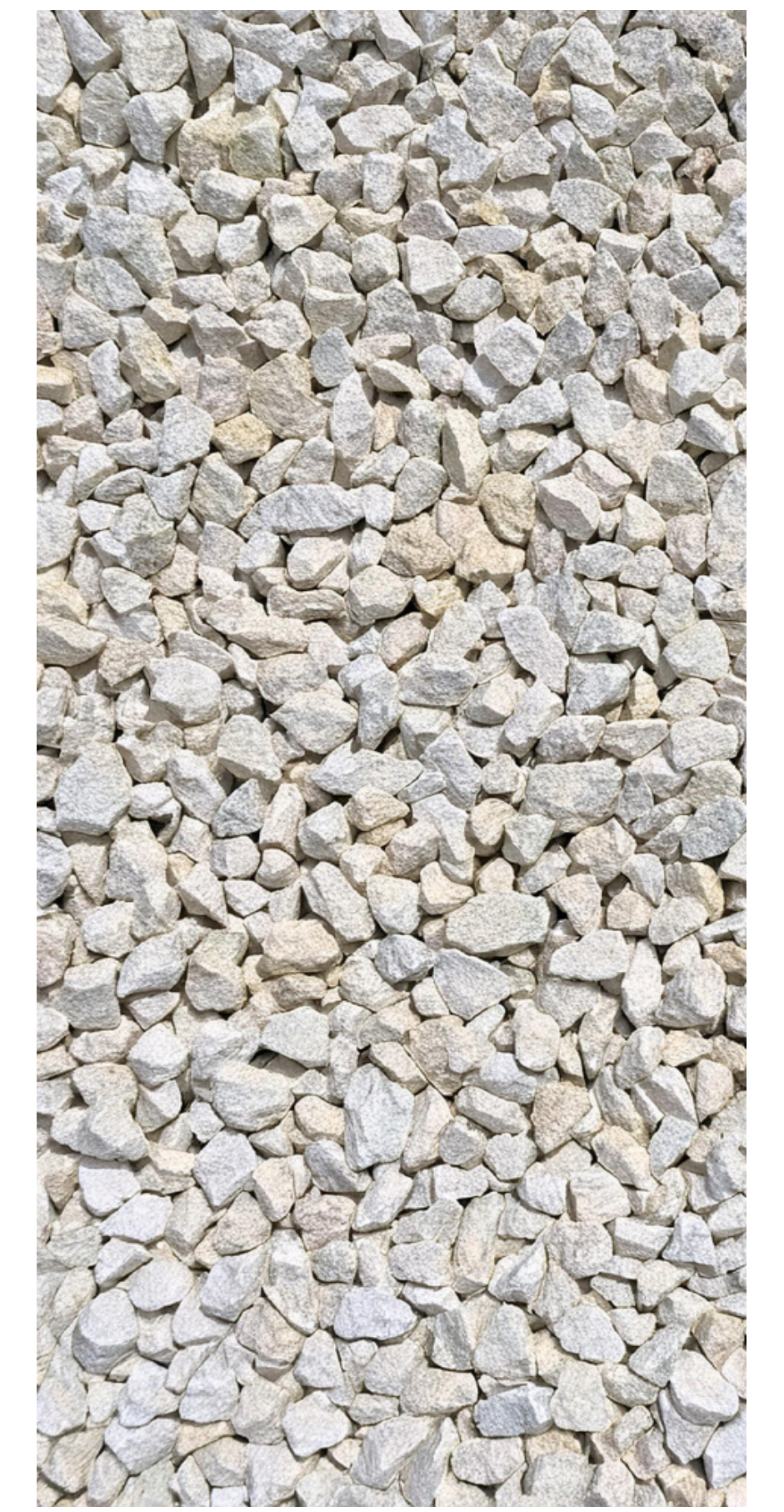
GRAVEL - ROOF TWO COURSE OF 1" AGGREGATE ADHERED ONTO ROOF MEMBRANE LIGHT TONE, COMPLY WITH COOL ROOF REQUIREMENTS
