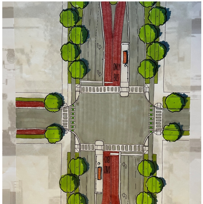
Figure 29: Proposed intersection plan for Fair Oaks considering a transit intersection approach
